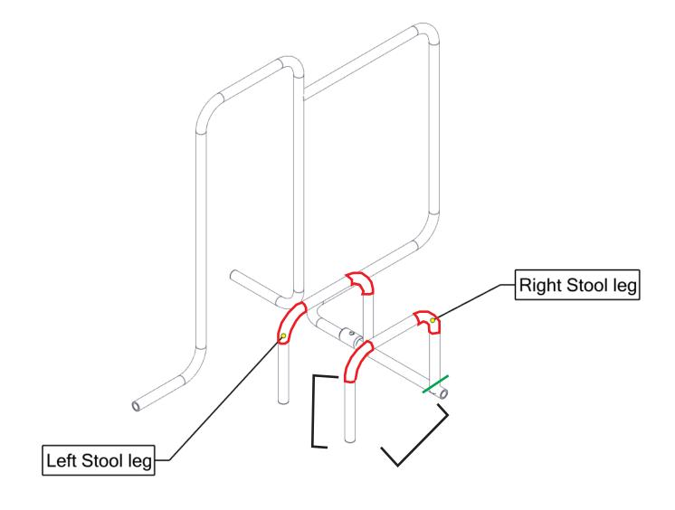
Bend the pipes so that they complete a half shape as shown in the diagram. After bending, cut one end to a depth of 22 mm. Then weld the **cut** end to the pipe as shown in the diagram. The distance between the pipes is 17 cm.
