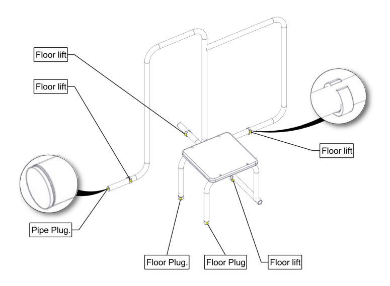
Pre-drill holes with a diameter of 5.5 mm in the marked areas and connect the printed parts according to the drawing.
