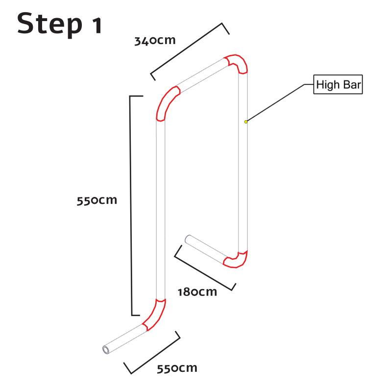
Take the pipe of length X and bend it using a 60 mm Beck pipe bender with a diameter of 22 mm and bend it to 90 degrees in the marked areas.
