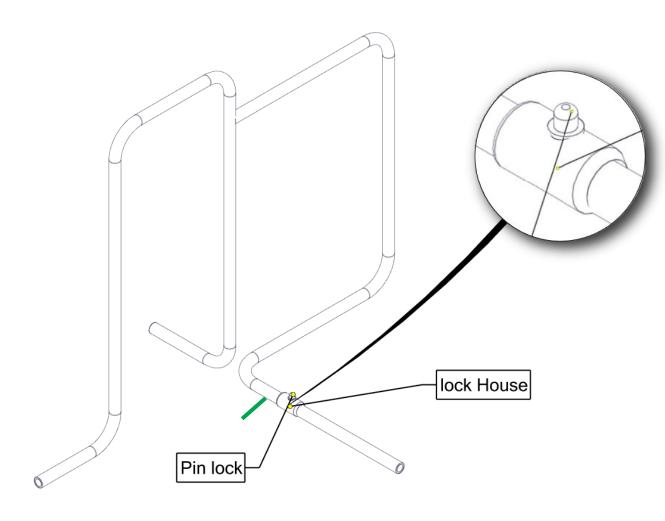
Take a 25 mm diameter pipe and cut a 65 mm long piece from it. Drill a 10 mm diameter hole 23 mm from the marked end.
