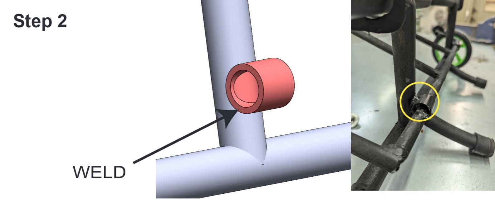
Cut two 22 mm long pieces from the 22 mm thick pipe and WELD to the area shown
