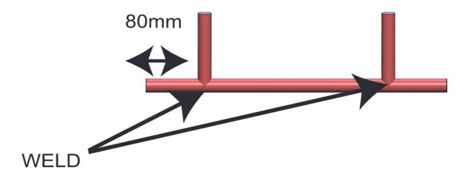
Cut two pieces of pipe 170 mm long from the 22 mm thick pipe and WELD to the central axis which is 470 mm long Make sure the pipes are connected at a distance of 80 mm from the end of the central axis
