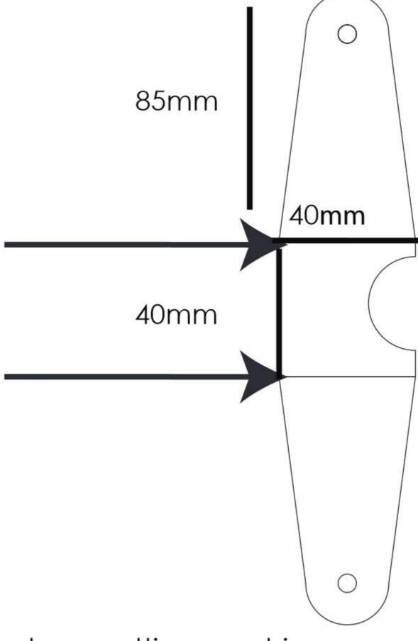
In order to create the front fork, you need to cut a 4 mm thick segment in a laser cutting machine in the following layout and bend it to 90 in the marked areas
