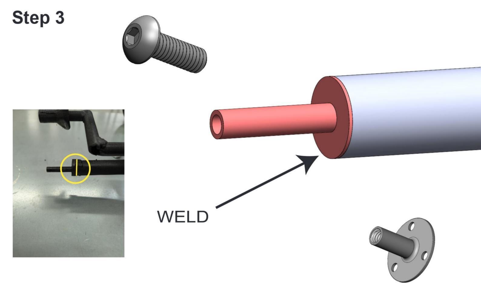
Make sure the shaft is concentrically connected
