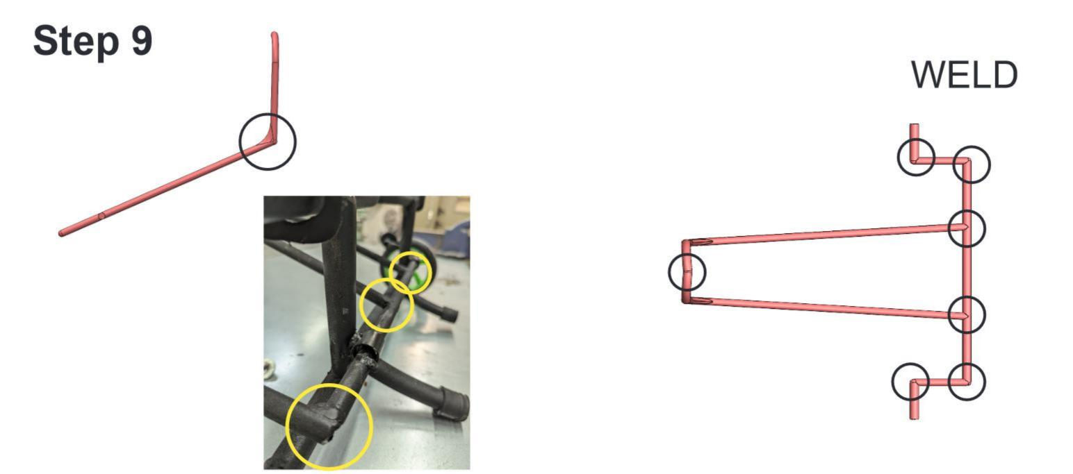
In order to make the brake, you need to take the 13 mm pipe and cut it according to the list of materials and weld it according to the description. It is important to \*pay attention
