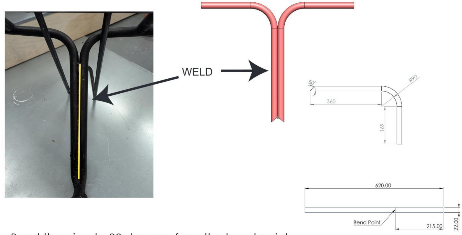
Bend the pipe to 90 degrees from the bend point 350mm from the bottom
